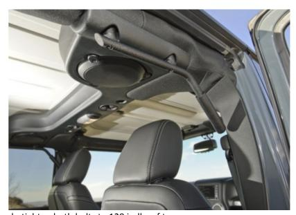
using a 5mm hex wrench, tighten both bolts to 120 in-lbs of torque.
