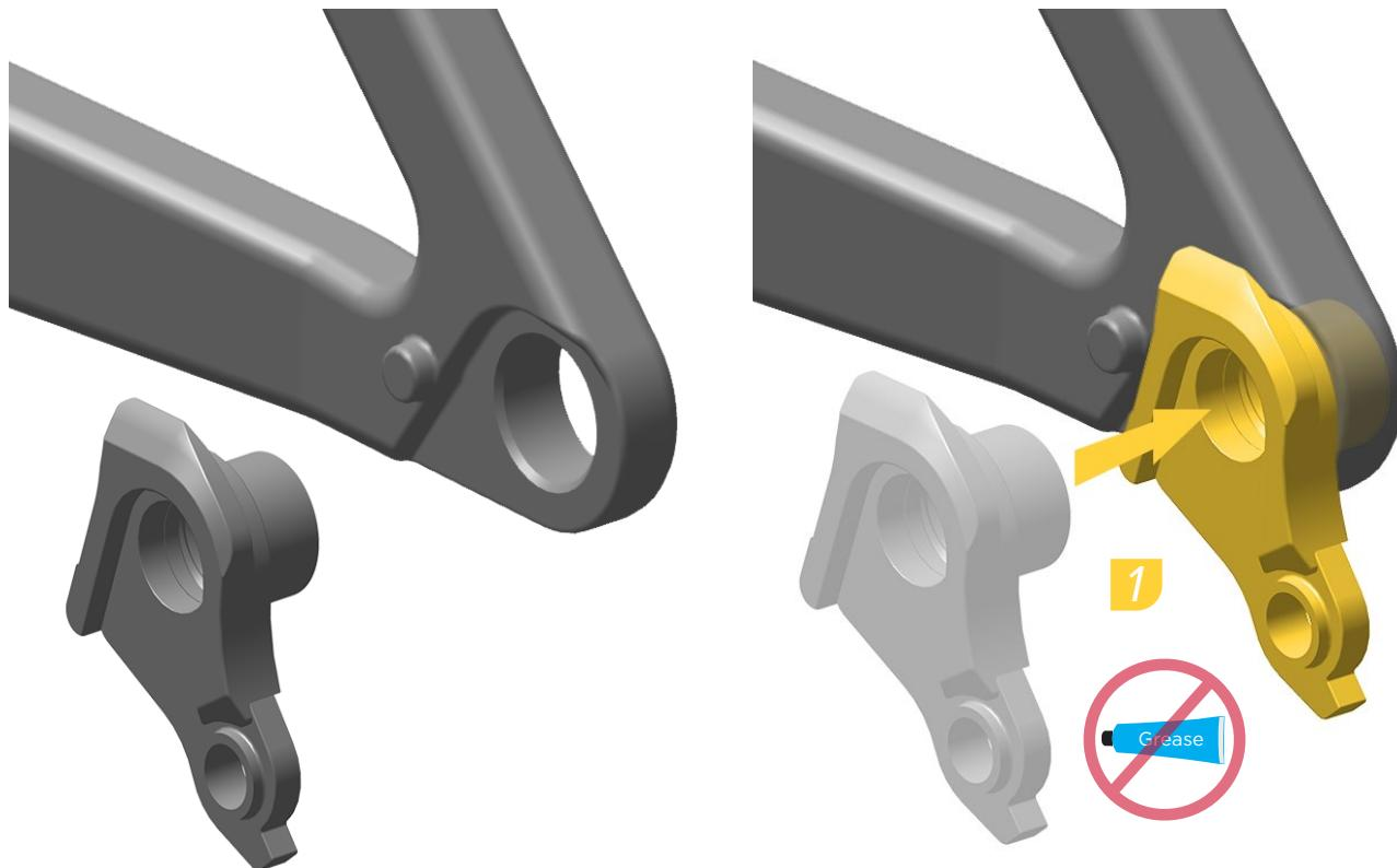
Install the UDH hanger assembly into the frame dropout.
