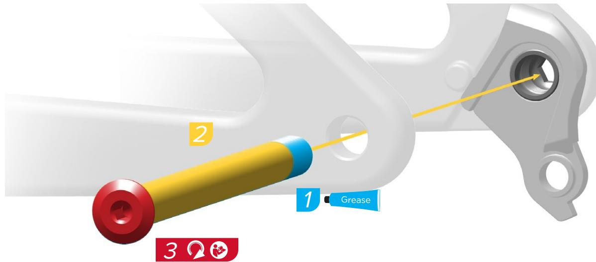
Apply grease to the thru axle threads before axle installation.
