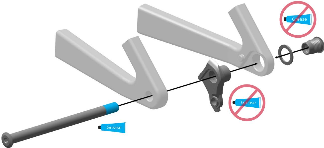
Apply grease ONLY to the thru axle threads.
