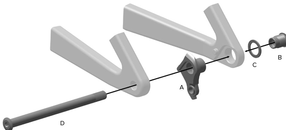
The UDH rear derailleur hanger (A) and UDH bolt (B) are only compatible with frames designed specifically for use with a UDH rear derailleur hanger.
