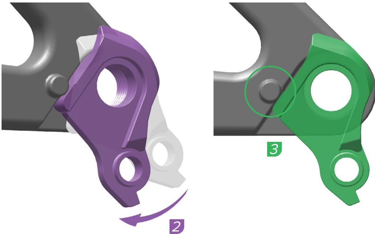
Rotate the UDH hanger forward until it is completely seated in the hanger pocket or contacts the rotational stop tab.
