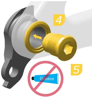
Install the frame-specific UDH washer. Install the UDH bolt through the washer and into the UDH hanger threads.
