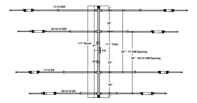
**Installation Notes:** Measure and mark each element location before installing the element (see diagram above). Install the elements *on top of the boom* and, once secured in place, rotate the traps so their drain holes face straight up (when the completed antenna is installed, it will be flipped over and the drain holes will face the ground). Refer to the Element Mounting Diagram below for details:
