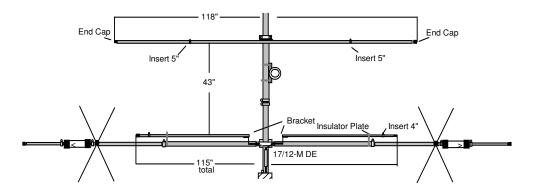
Important Note: Prior to installing the MA6B on a mast, check all hardware and worm clamps to confirm everything is properly aligned and tight. Also, check trap orientation -- drain holes must face the ground when the antenna is flipped over and installed on the mast.
