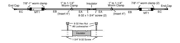
**Installation Notes:** Insert the insulator attachment screws in same direction and tighten securely (these screws will become the connection points for the feedline). Insert EB tubes <u>4</u> inches into EA tubes. Install all traps with the arrow pointing away from the boom. Install end caps on EC tubes.
