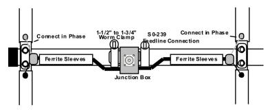
**Installation Notes:** Orient the MN6B junction box so the SO-239 faces toward the center of the antenna. Connect the two feed harnesses in phase (red leads on same side). Position the junction box so any slack in the two feed cables is equal in both directions. After securing the box with a worm clamp, disconnect the harness from the 17/12-meter element (it will be reconnected in Step-9 after the 6-meter driven-element brackets are placed in position).
