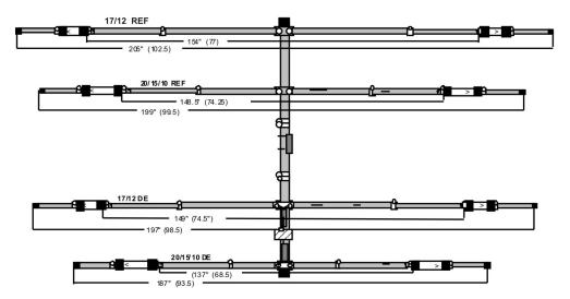
**Step-7. Install X-hats on the HF elements:** To avoid damaging the X-hat rods, the antenna must be elevated on saw horses or similar supports. Install X-hats using the components listed below:
