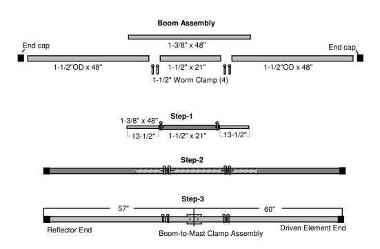
**Installation Notes:** Assemble boom tubes as shown above. Install end caps and secure all worm clamps tightly to prevent the boom sections from rotating out of alignment when elements are attached. Before installing the mast-to-boom clamp, measure off and mark the boom at 57" (see below):
