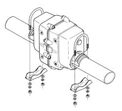
Be sure to leave enough slack in both the elevation control cable and the coaxial cable feedline around the azimuth rotator so the antenna can rotate  $450^{\circ}$  without straining the cable or feedline.
