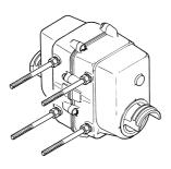
2. Slip an 8 mm flat washer over each installed stud bolt, and then the pipe clamps. Place another flat washer and then a spring washer over the end of each stud bolt, and start a nut on each to hold the hardware in place.
