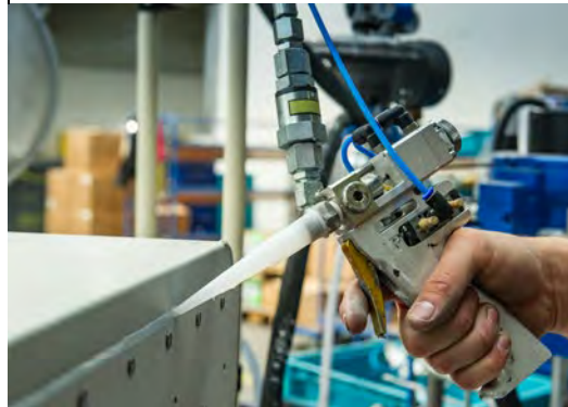
7 Application of the silicone seam with the dosing device
