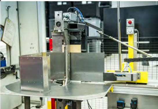
2 Bending the outer shell in the production cell
