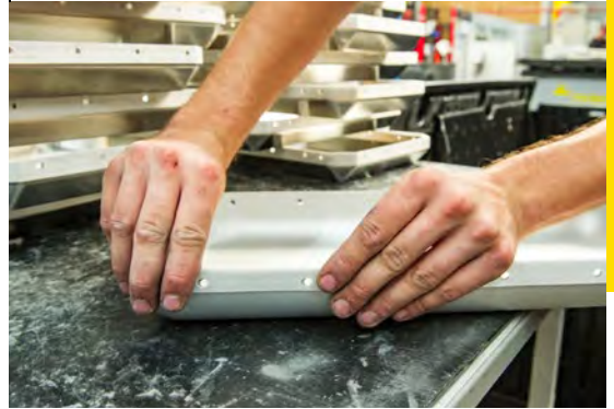
6 The base of the ZEGA Evo is sealed with a silicone sealing tape
