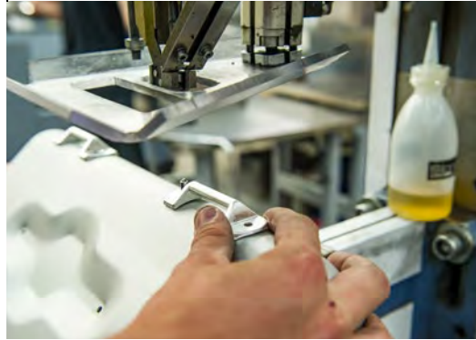
4 Riveting eyelets onto the lid of the ZEGA Evo
