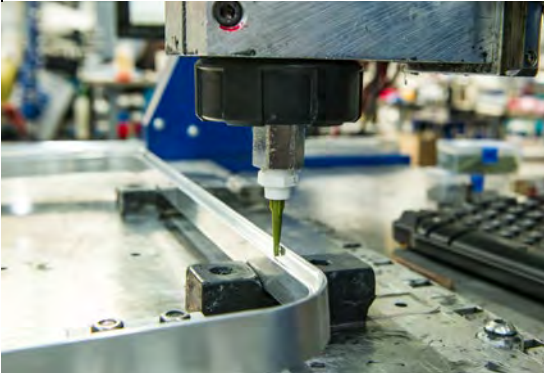
5 Automatic dosing of adhesive
