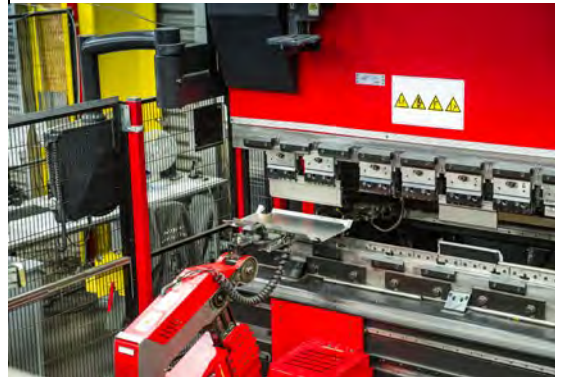
3 Automated bending of base and lid (in this case a BMW pannier)
