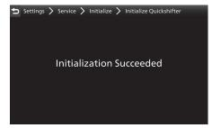
If the display shows the message that "Initialization Failed", check the mounting conditions of the quick shifter, then restart the initialization again.
