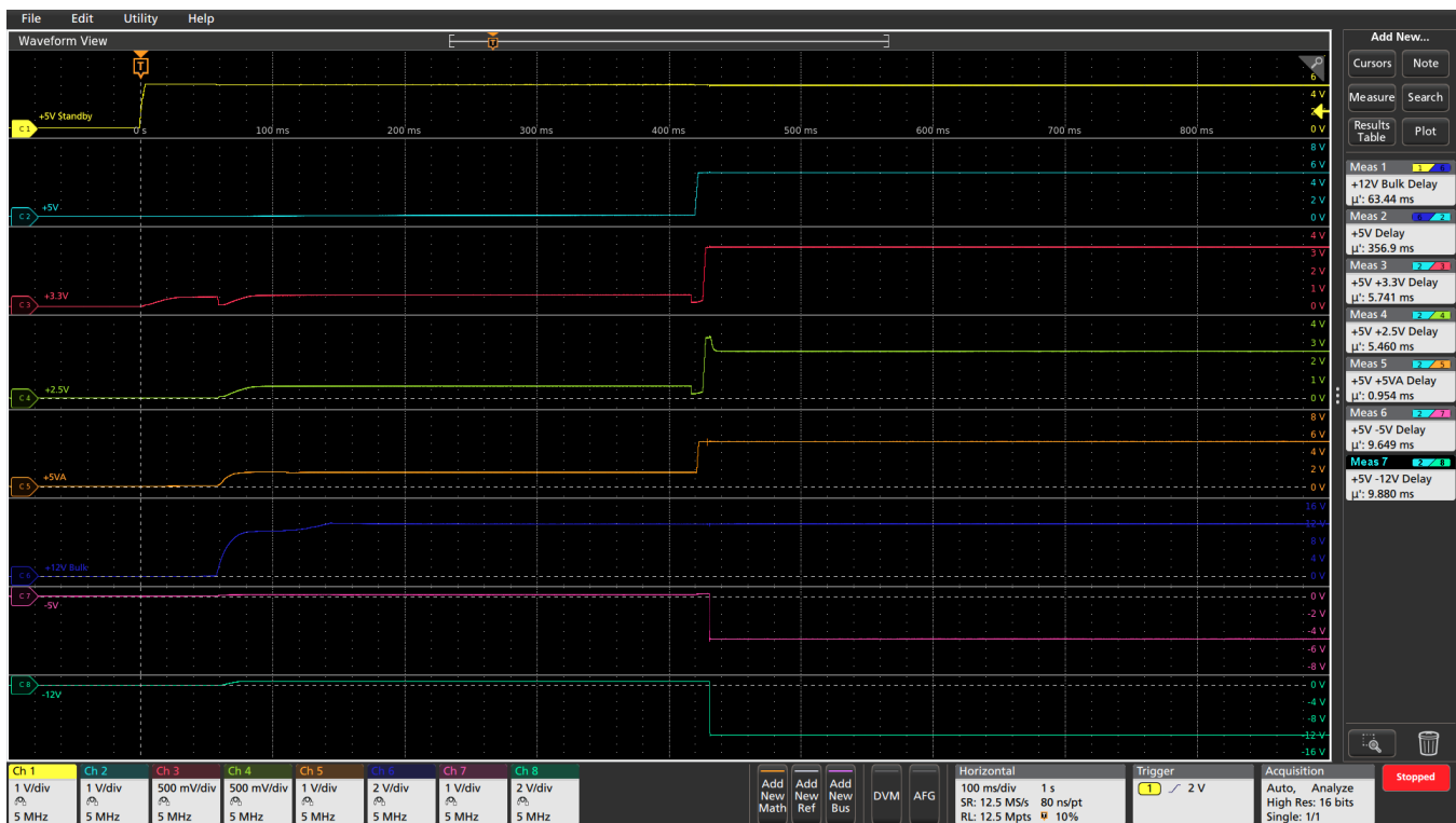
Figure 19: Using automated measurements to characterize power supply bring up.
