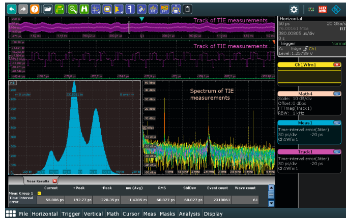
Detection of frequency interference within a clock signal: tracking of TIE jitter; histogram and FFT analysis of track curve.
