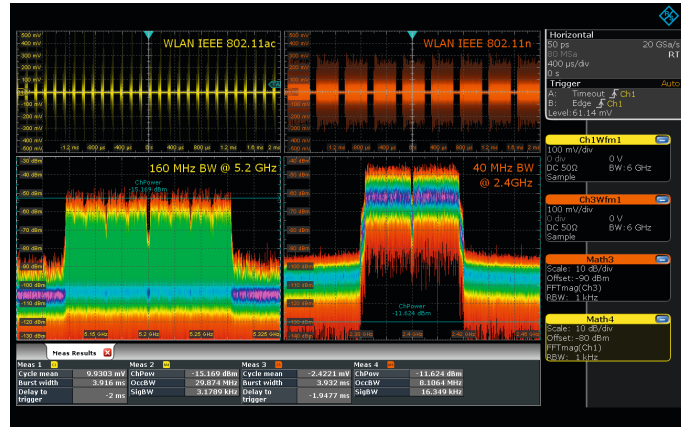
R&S®RTP multichannel frequency analysis of a WLAN IEEE802.11n and 11ac MIMO signal.
