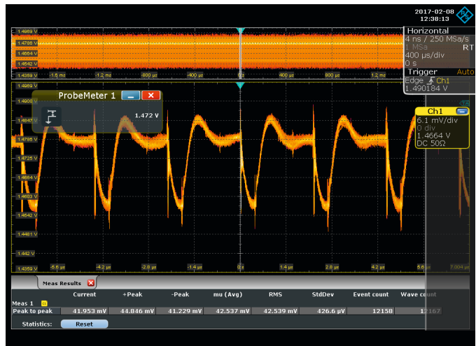
Accurately verify DC level and power supply load response during initialization of a DDR memory with the R&S®RT-ZPR power rail probe and its integrated high-precision R&S®ProbeMeter.
