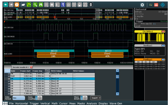
The digital channels are ideal for triggering and decoding low-speed serial interfaces such as SPI.
