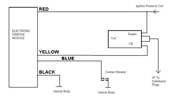
If you cannot tell which wire leads to the points, disconnect both low voltage wires from the coil. One should have supply volts present with the ignition on (coil power, measure with DC voltmeter), and the other should be open and closed circuit as the points are opened and closed (points wire, measure with ohm meter).
