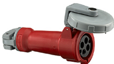
Watertight IEC Pin and Sleeve Connector, 4P5W, 30A 3PH120/208V
