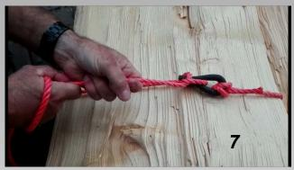
Attention: To open the connection, put the wood bundle with Knoti in the upper area so that the rope connection loses some tension (this is the case with dried wood anyway). Now pull the rope end in the same direction as when straining, i.e. exactly in the direction of the conical pin. If you pull skew to the side or if the tension is too high, the connection cannot be opened! Turn the bundlea little or pull out a log to the side!
